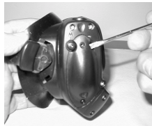
Fig. 115 - BATTERY COVER REMOVAL
