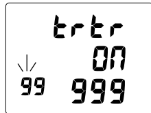
Fig. 37B - SET LINK CODE (SERIAL NUMBER)
