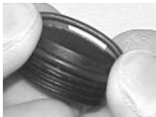
Fig. 119 - TRANSMITTER O-RING INSTALLATION
