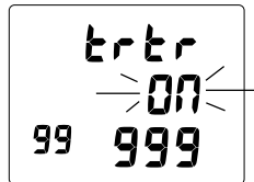
Fig. 37A - SET LINK CODE (ON / OFF)
