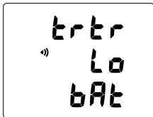
Fig. 3 - TRANSMITTER LOW BATTERY
