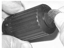
Fig. 118 - TRANSMITTER BATTERY COVER REMOVAL
