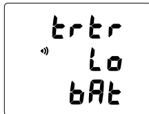
Fig. 16 - TRANSMITTER BATTERY LOW
